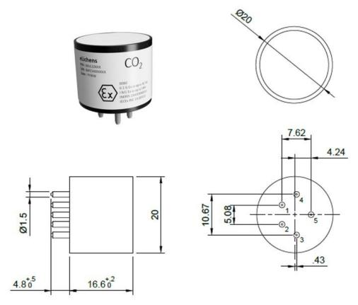
All dimensions are in millimeters [mm]
